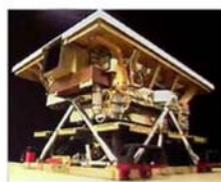
Visible and Infrared Mapping Spectrometer
